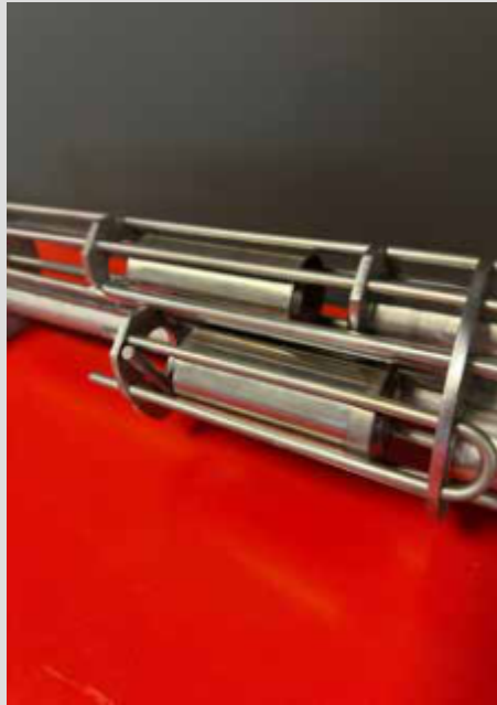
Possibility for zero separation distance for the two upper alarm levels.
