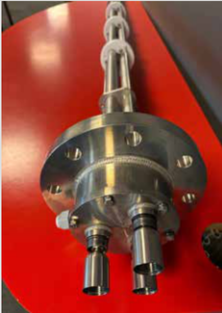
Level switch with new design for individual alarm level test.
